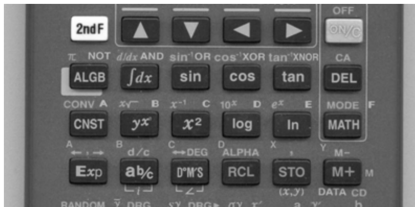
Figure 5.3 Keys used to calculate an exponential value using a typical scientific calculator
